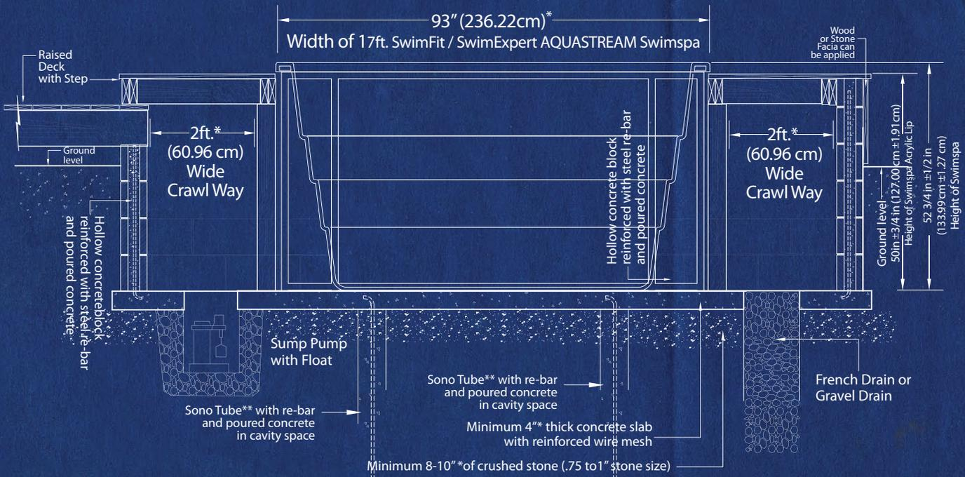
\*\* Sono Tubes only required in installations that are in regions that experience freezing and thawing.
