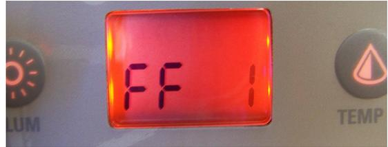
The display will show FFxx, with "xx" representing the number of cycles per day. Use the arrow keys to adjust the frequency. Use the Light Key to jump to the next parameter, economy mode (EP)
