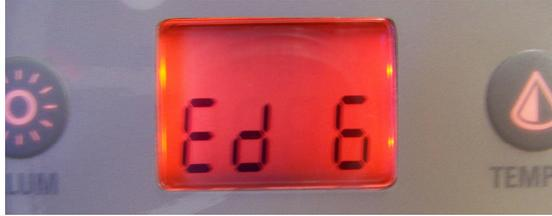
The display will show Edxx, with “xx” representing the duration in hours of the economy mode. Use the arrow keys to adjust the hour. Use the Light Key to jump to the next parameter, temperature unit.
