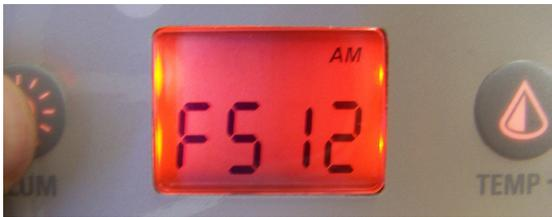
After you have programmed the clock, the next parameter is the filter cycle start time. The display will show FSxx, with “xx” representing the starting hour of the cycle. Use the arrow keys to adjust the hours. Use the Light Key to jump to the next parameter, filter duration (Fd).
