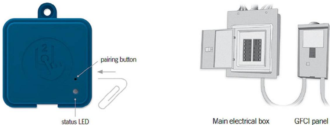
If you need to replace a transmitter or pair your transmitters again, power up the home transmitter and press on its pairing button with a paper clip. The status light of the transmitter will blink yellow.
