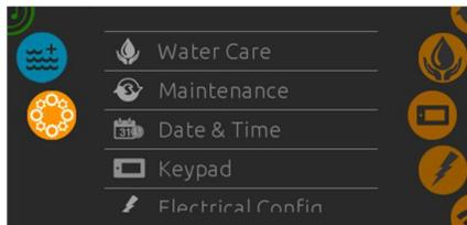
Use the icon keys to scroll up and down in the list. To select an option, press the text.
