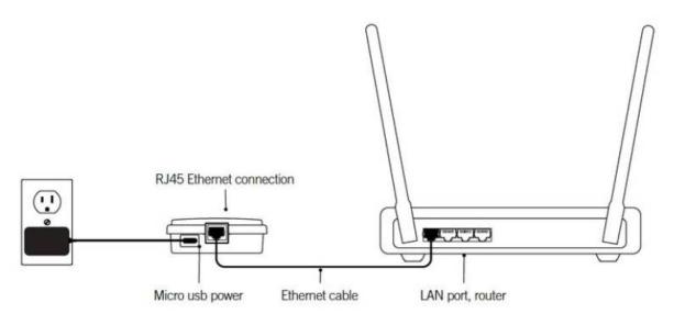
Simply connect the Ethernet cable into the RJ45 port of the in. touch 2 home transmitter and in one of the available LAN ports on your router. To power up the home transmitter, plug the provided wall outlet charger to a 120V (North American model) or 220V (European model) household supply and connect the USB cable to the wall outlet and the home transmitter.
