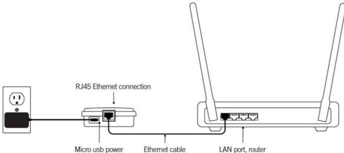
Simply connect the Ethernet cable into the RJ45 port of the in. touch 2 home transmitter and in one of the available LAN ports on your router. To power up the home transmitter, plug the provided wall outlet charger to a 120V (North American model) or 220V (European model) household supply and connect the USB cable to the wall outlet and the home transmitter.
