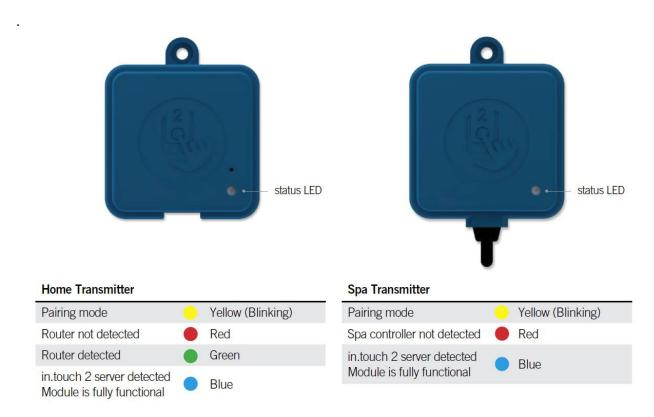
When the LED status is blinking (blue, green or red) this indicates that the communication between the EN module and the CO module it not established.
