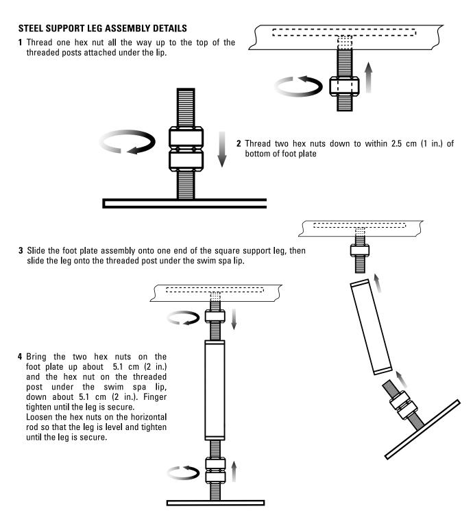
5 After the swim spa is filled with water, the legs can now be adjusted as necessary from either the top or bottom with a wrench to ensure that the walls are straight and level. See section FILLING, CHECKING & STARTING YOUR SWIM SPA
