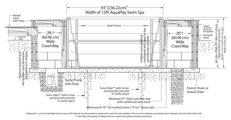
Cross Section End View of 2020 12fX AquaPlay Swim Spa Full Inground Installation...
