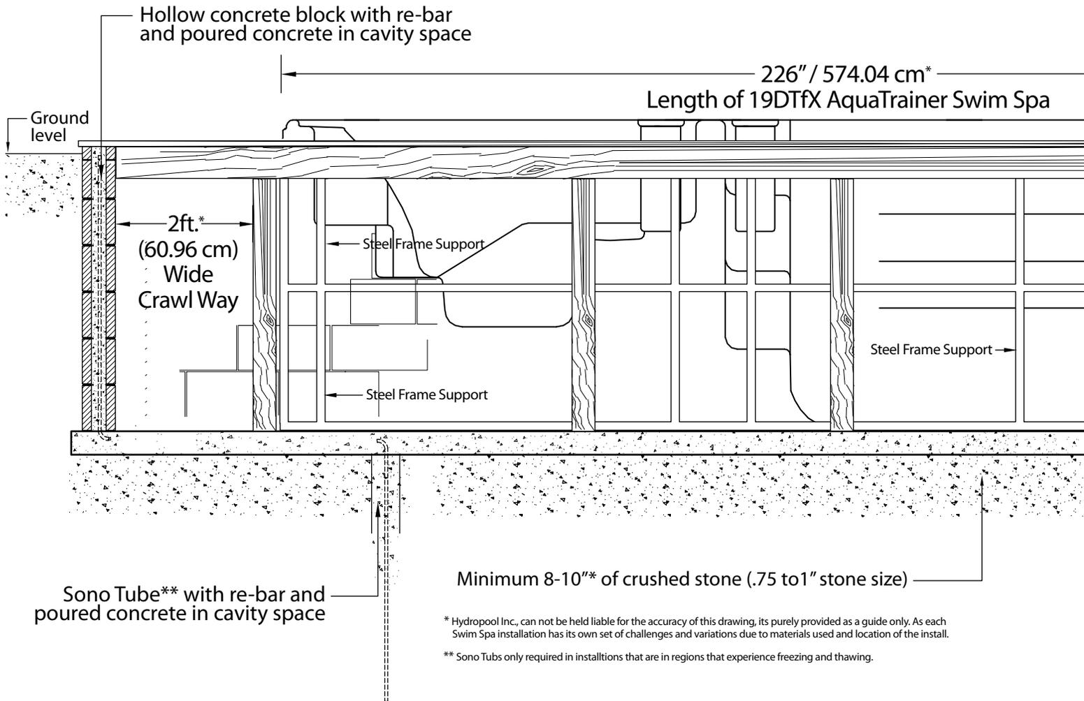
\*Hydropool Inc., can not be held liable for the accuracy of this drawing, its purely provided as a guide only. As each Swim Spa installation has its own set of challenges and variations due to materials used and location of the install.
