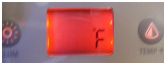
Water temperature can be displayed in either Fahrenheit (°F) or Celsius (°C). The display will show °F or °C. Use the arrow keys to change the setting. Use the Light Key to save all the parameters.
