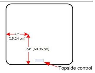
FIGURE 1: ELECTRICAL CONDUIT LOCATION
