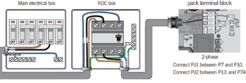
Electrical wiring: European model in.ye – in.yt Main electrical box RDC box
