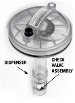
Built in dispenser: if your Hydropool hot tub was ordered with the optional built in bromine/chlorine dispenser, (located in the lid of the cartridge filter housing), refer to section CARTRIDGE FILTER for details on removing and re-installing the lid. Once the filter lid is removed, you'll notice a clear 2.5 cm (1") diameter tube extending from the bottom of the lid. Unscrew the check valve
